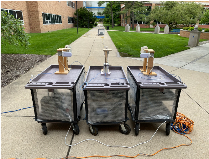
Fig. 4. Photograph of the distributed phased array. Antenna masts are placed along the far edge of the carts. On the far side of the mast are 10-dBi log-periodic antennas, on the near side are 8-dBi log-periodic antennas on the secondary nodes while the primary node has an omnidirectional commodity dipole antenna. In front of the array near the ground is the triggering antenna which also used an 8-dBi log-periodic antenna; similar 10-dBi and 8-dBi log-periodic antennas were included on the receiver cart located \sim 17 m downrange for receiving beamforming and triggering waveforms, respectively.
