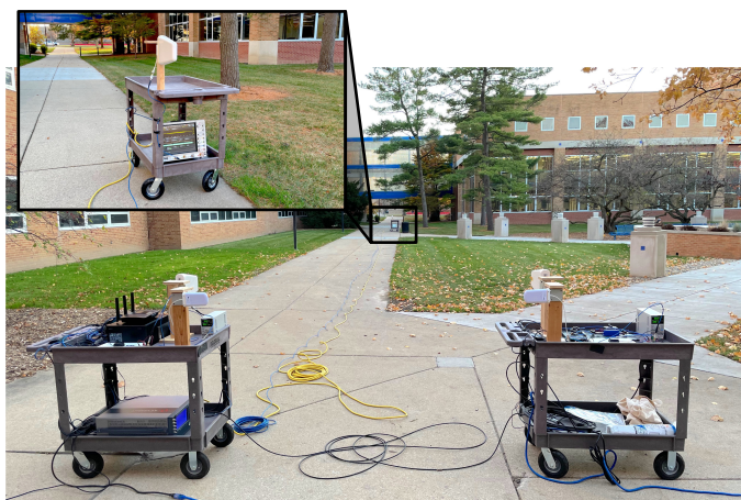
Fig. 2. Experimental configuration of the distributed beamforming system in a fully enclosed courtyard. Node 0 is on the left and node 1 is on the right, separated by 2.1 m. The ranging target, shown in the inset is located 41 m downrange, below the blue walkway. A 20 GSa/s sampling oscilloscope was used to digitize the waveforms at the carrier to estimate time delay, phase, and coherent gain at the beamforming location.
